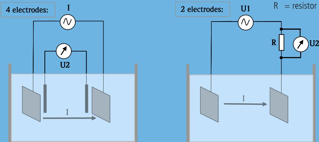
AC excitation is recommended to reduce degradation of the electrode and electrolyte
