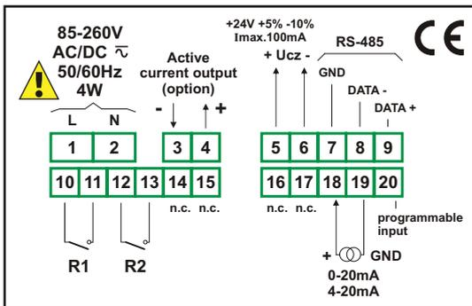
version with 4-20 mA output and two relays
