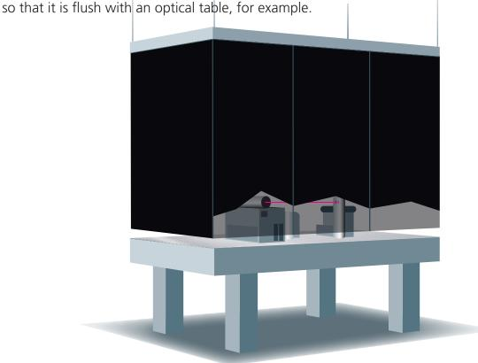
Single, mobile laser safety screen in a metal frame – fitted with laser safety curtain, solid metal sheet or laser safety glass.
