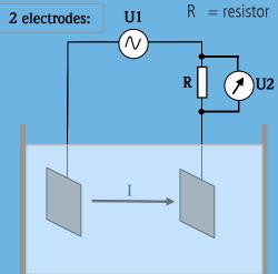
AC excitation is recommended to reduce degradation of the electrode and electrolyte
