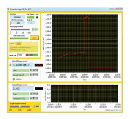
The LabView based free software "DigiLog" is a tool for displaying and logging of irradiation and temperature data generated by the sglux digital UV sensors. The measurements and the data appearance can be customized. The output data is logged in a file.
