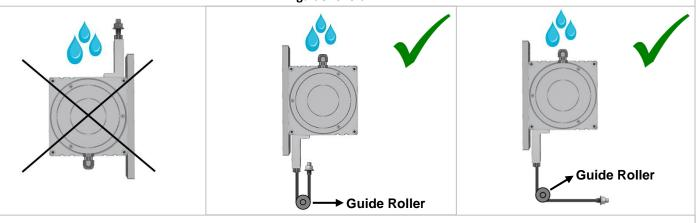
4. The wire should not be pulled in angular. If needed, please use guide rollers.
