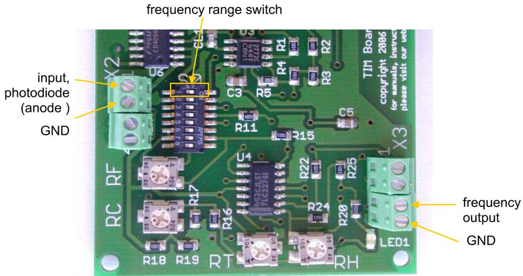
Fig. 3: Current-to-Frequency Converter input, output and switches
