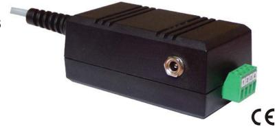
The **SRS-2/4-Z45** converter module is used to connect MASTER devices with a RS-232 port to a RS-485 bus. The module supports devices, which control Tx switching using the RTS signal and devices, which do not control Tx switching using the RTS signal (Tx switching is then fully automatic). For example, a suitably programmed PC computer can function as the system MASTER device.
