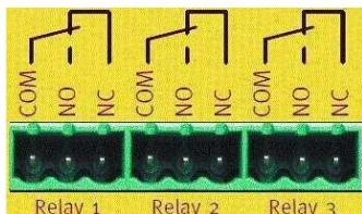
Three potential-free relays can be used for process control.
