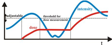
In the second example the dose measurement is finished with falling under the intensity threshold. The reset delay keeps the value on the display. At exceeding of the threshold a new dose is generated. The generation of single doses is used if the dose stop condition is activating a pump or a transport of a good (see below). For each irradiated good or segment a dose is calculated.
