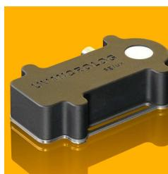
The **UVMICROLOG** is designed for logging of ultraviolet radiation, temperature, pressure and acceleration. Sophisticated microcontroller technology and low noise SiC TOCON based UV detectors allow up to 3 months of permanent measurement and logging without battery charging. The unit can be mounted with a belt or screws.
