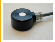
The **UVFLASHCON** is designed for measuring short pulses of UV flash lamps. It gives an output level of 5V as long as the UV flash lamp intensity is higher than a configurable threshold. If no flash intensity is exceeding the threshold for a choosable time, the output level falls to 0V.
