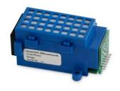
Infrared gas sensor using dual beam technology, with measurement and reference channel, for monitoring room air and process control applications. Integrated evaluation electronics for drift and temperature compensation.
