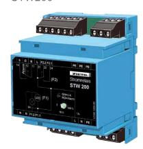
Current-relays STW200 monitor AC-currents for falling below an adjusted limit. The ranges 12 ... 120 mA and 0,1 ... 1 A allow the monitoring of LED-Lamps as well as incandescent lamps in obstruction lights.
