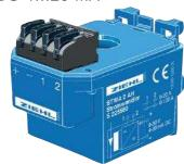
The STWA2AH is a measuring transducer for AC currents 0...100 A, divided in 2 ranges 0...20 A and 0...100 A. Multiple loops of the conductor through the transformer reduces the measuring range correspondingly (for instance to 0...5 A with four loops).
